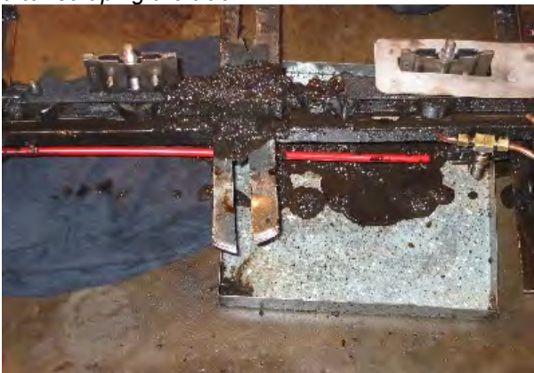
Below: Picture of carbon sludge found after scraping the track.
