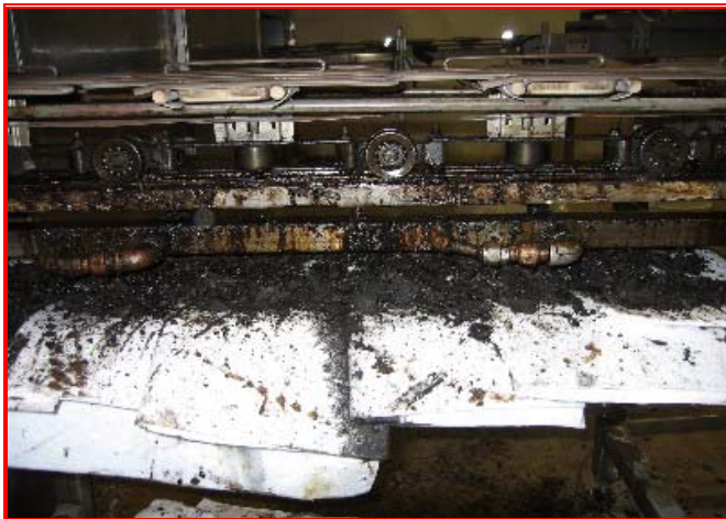
Carbon Debris Removed before converting to HT-2000™ by using CC-2208 Carbon Clean
