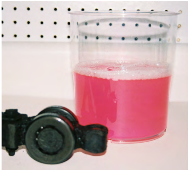
SEVERE CARBONIZED ROLLER SOAKED IN SUPREME CLEAN FOR 5 DAYS.
