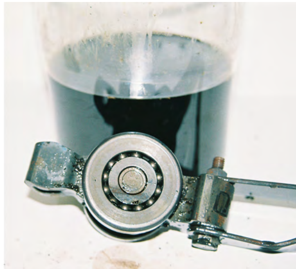
ROLLER CLEANED AND ROLLER BALL BEARINGS FREE FROM CARBON.
